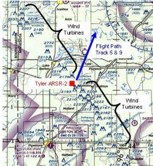
Figure 28. Location of wind turbines with respect to ARSR-2 radar at Tyler
