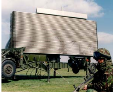
Figure 23. Commander AR327 - Type 101 air defense radar
